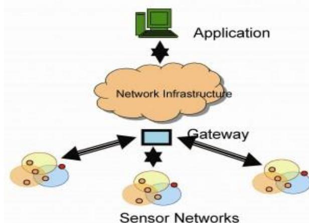
Figure 1.1 Architecture of sensor networks
