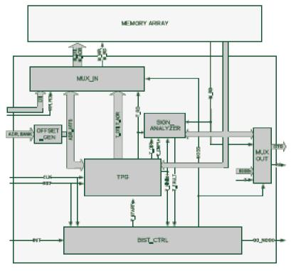
Fig 2. Architecture of the memory module with BIST controller
