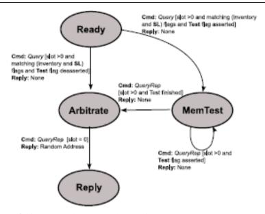
Fig.1 Transponder access scheme with concurrent test state
